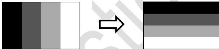
Figure 2 – “Typical” image used for power consumption measurement
